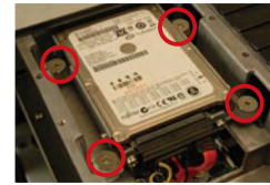
HDD install with Anti-shock buffer rubber enhances protection performance.
