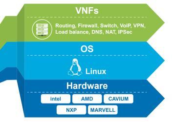
Universal CPE (uCPE) is one of the most compelling use cases of Network Function Virtualization (NFV) currently attracting the interest of hosted service providers. uCPE provides a remotely manageable platform on which hosted service providers can easily deploy, modify or delete VNFs over Wide Area Networks (WAN).
