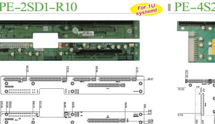
Mounting holes compatible with PCI-4S
