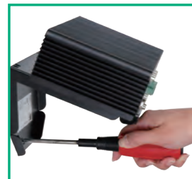
2: Select the position to mount stand kit
