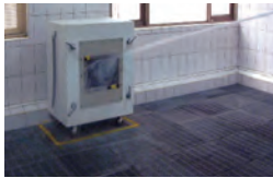
IEI's LCD products are front sealed and tested in the certified house chamber under UL's Witnessed Test Data Program (WTDP).
