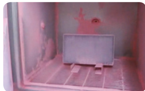
Test for protection against dust
