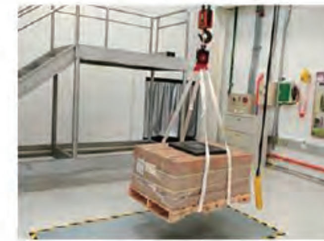
Pallet Package Drop Test
