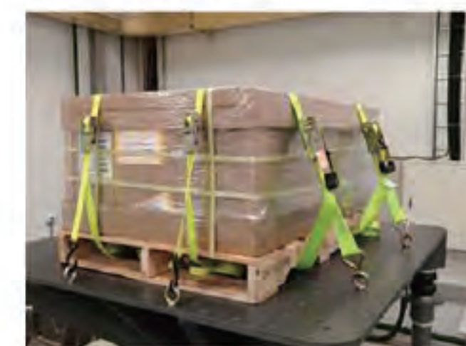
Pallet Package Vibration Test
