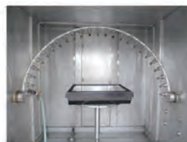
Anti-Water IP-X4 Testing
