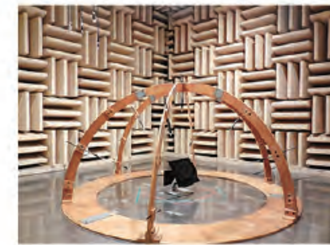
Acoustic-Sound Power Test
