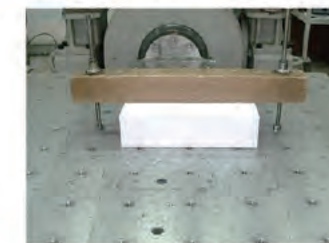
Single Package Vibration Test
