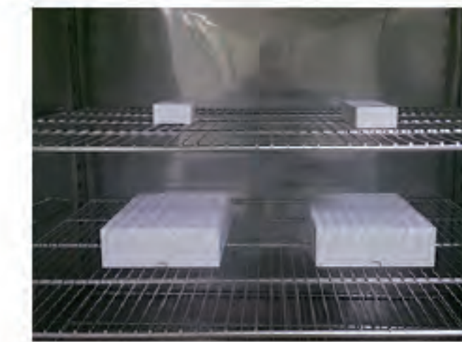
Package Temperature Humidity Test
