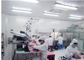
Control room particle measure result: Class 10000
